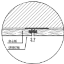
double female groove joint with allowance joint
